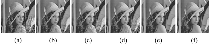
Fig. 9. Reconstructed images with (a) P_f = 0.2 , P_d = 0.5 , PSNR = 22.4303 and N_{re} = 800 ; (b) P_f = 0.2 , P_d = 0.7 , PSNR = 22.7172 and N_{re} = 800 ; (c) P_f = 0.2 , P_d = 1 , PSNR = 40.3389 and N_{re} = 545 ; (d) P_f = 0.1 , P_d = 0.5 , PSNR = 22.5194 and N_{re} = 800 ; (e) P_f = 0.1 , P_d = 0.7 , PSNR = 24.6407 and N_{re} = 800 ; (f) P_f = 0.1 , P_d = 1 , PSNR = 40.349 and N_{re} = 498 .
