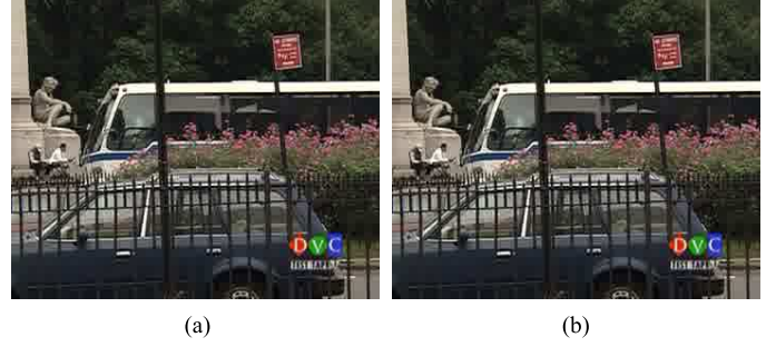
Fig. 10. (a) Imperfect channel sensing with P_d = 0.8 , P_f = 0.2 , PSNR = 15.3170 dB and N_{re} = 3059 (b) Perfect channel sensing with P_d = 1 , P_f = 0 , PSNR = 15.6711 dB and N_{re} = 889 . (a) Imperfect sensing. (b) Perfect sensing.
