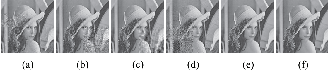
Fig. 13. Reconstructed images with (a) QAM, m = 1 , PSNR = 18.8928 and N_{re} = 410 ; (b) HQAM, m = 1 , \alpha_0 = \alpha_1 = 1 , PSNR = 21.3205 and N_{re} = 410 ; (c) HQAM, m = 1 , \alpha_0 = \alpha_1 = 2 , PSNR = 22.4221 and N_{re} = 410 ; (d) QAM, m = 2 , PSNR = 19.1760 and N_{re} = 396 ; (e) HQAM, m = 2 , \alpha_0 = \alpha_1 = 1 , PSNR = 35.6625 and N_{re} = 400 ; (f) HQAM, m = 2 , \alpha_0 = \alpha_1 = 2 , PSNR = 37.8730 and N_{re} = 366 .
